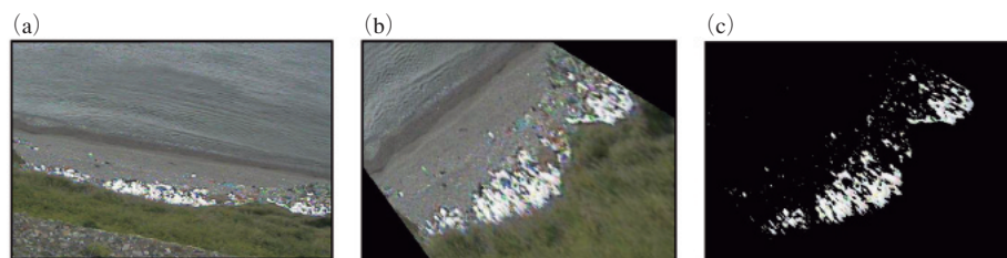
Fig. 2 Photographs taken by webcam 1: (a) the original photograph taken by webcam 1, (b) the photograph after applying the projection transformation to (a). The panel (c) is the lightness map on which pixels with the lightness greater (lesser) than the threshold value in (b) are colored in white (black).
